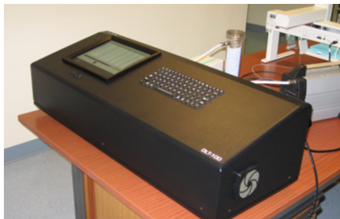
The DT-100 liquid water stable isotope analyser. Autosampler, vacuum pump and Drierite column are shown in the background.
